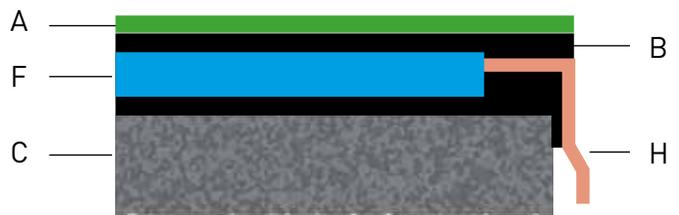
Figure 5 presents a cross-sectional example of a possible covering solution at the front edge of a balcony.
