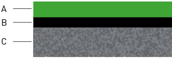
Figure 1 shows a cross-section of a balcony floor structure. The covering (A) has been fixed to the concrete floor (C) with ElaProof (B). In this example, the covering is a flexible plastic sheet.
