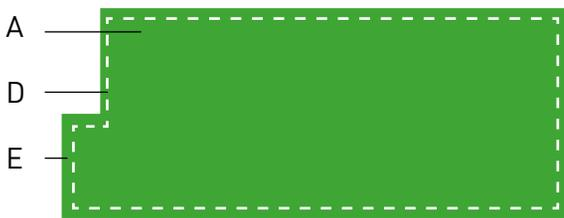
Figure 2 presents a balcony floor covering (A), cut to size in the factory, from above. The broken line represents the layer of reinforcing material (D) installed under the covering. The edging (E), which is folded upwards against the wall from the concrete surface, is also shown.
